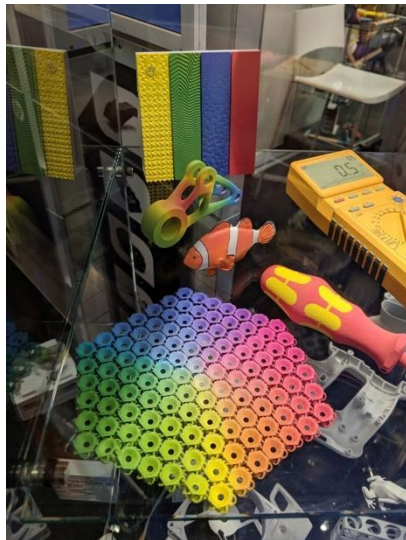
Figure 6: Possibilities of multicolour printing with MJF. Source: CC BY-SA 4.0 by L. Müller/Hochschule Düsseldorf.
