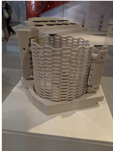
Figure 1: Part fully made out of sand. Source: CC BY-SA 4.0 by L. Müller/Hochschule Düsseldorf.
